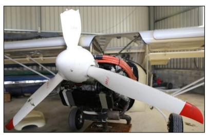
Photo No. 1: Propeller blade damage
